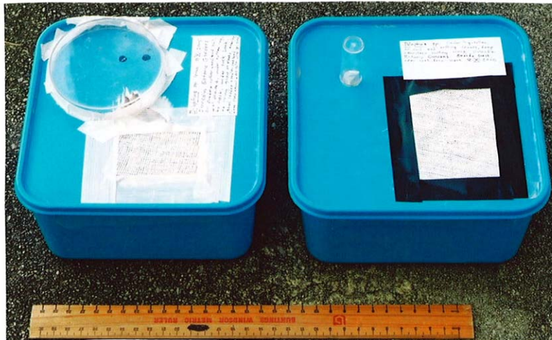
Figure 1. Left. Standard, 2-litre plastic ice cream container showing inverted Petrie dish stuck to lid, and below it, two holes for entry of emerging adult March flies. Right, container with inverted tube to retain emerging adult March flies. Scale: ruler marked in cm.
